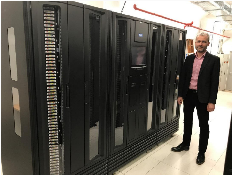
Bojan Kosi, Head of the Mediateka team, standing next to the Qualstar XLS robotic LTO library, managed by XenData.
